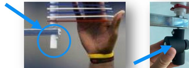
**Step 2:** Use the screw and washer to attach the Dashr | Jump ball-joint coupler.
